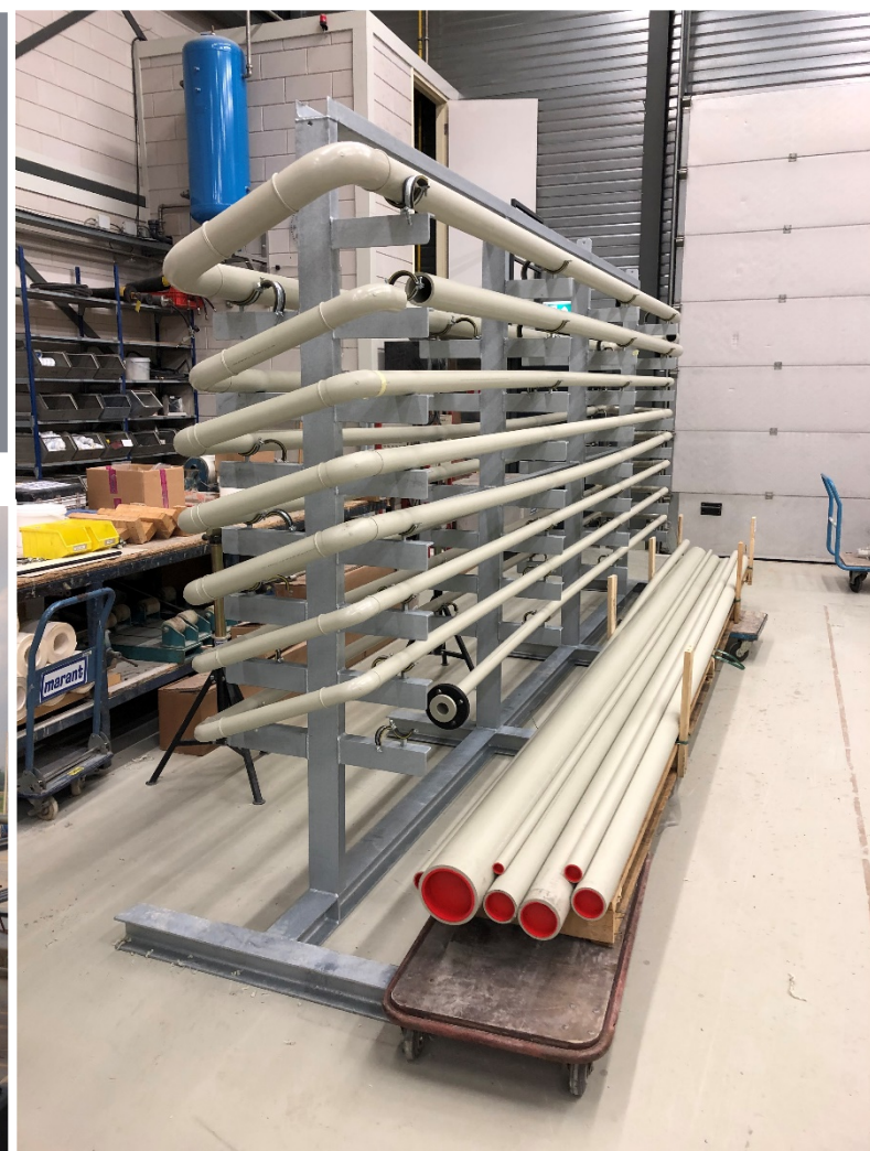
Smaller CPR under construction. This one was designed for a flow rate of 10 m 3 /h. The material of construction is PP.
