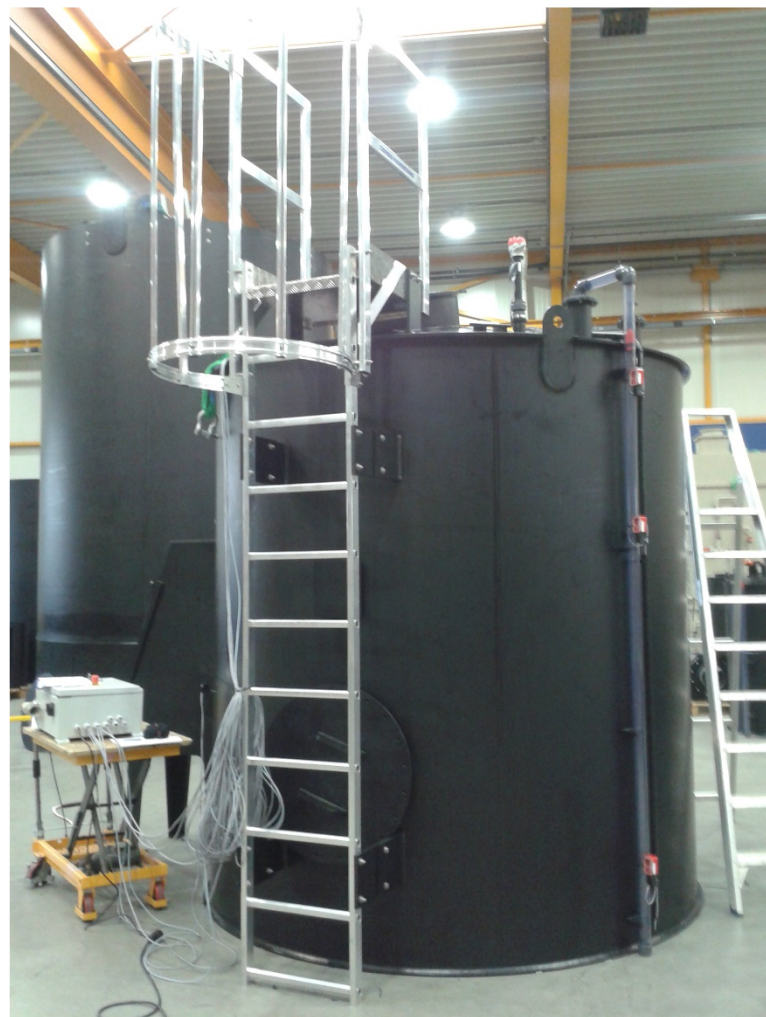
HDPE chemical storage tank during FAT testing
