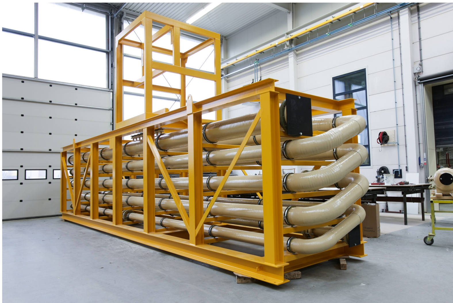
Large CPR with GRE-CST (conductive) pipes. This CPR is part of a produced water treatment plant with a capacity of 250 m 3 /h
